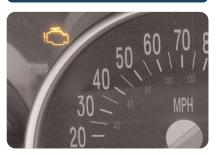
If the Malfunction Indicator Light is Flashing: When it is safe to do so, stop the vehicle and turn the engine off. Wait 10 seconds and restart the engine. If the light stays on steadily, see the steps below. If the light continues to flash, follow the previous steps and see your dealer for service as soon as possible.
